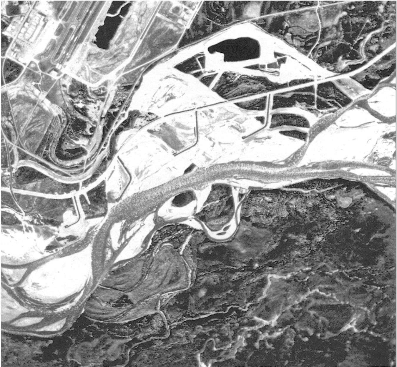
Figure 3-20. Tanana River at Fairbanks showing in-river levee and groins
