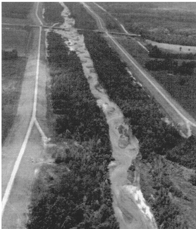
Figure 3-21. Side bar deposition and sub-meandering in straight channel
